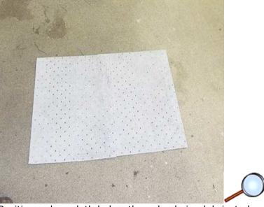
2. Position a drop cloth below the valve being lubricated.
