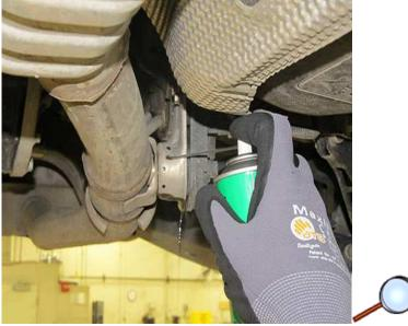
3. Apply DRY SLIDE Multi-Purpose Dry Lubricant, P/N 1052948 (in Canada, use 89021511), into the valve by inserting the nozzle into the slot on the valve. Liberally apply a generous amount of the lubricant.
