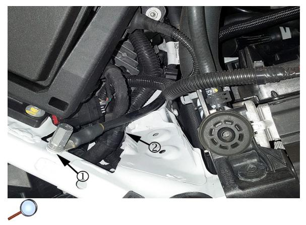
2. Remove the battery negative stud (1) to gain access to the harness junction (2).
