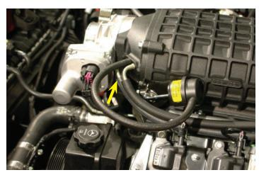
135. Tie the PCV, Brake Booster, and Bypass hoses together loosely with a zip tie as shown.
