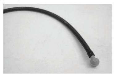
133. Depending on the car, install the check valve or sensor with hose at the brake booster as shown. Route the hose laterally toward the engine and turn it forward to parallel the PCV hose just installed.
