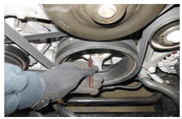
51. This picture shows that the pins are behind the surface where the pulley bolt will touch.
