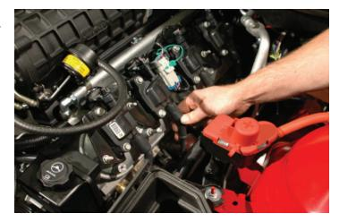
121. Plug in the electronic throttle body connection on the driver side of the throttle body.
