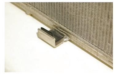
77. Attach one strip of the adhesive backed foam to the inside-upper edge of the heat exchanger, overlapping the rubber strips as shown.
