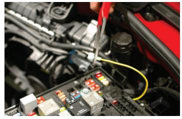
184. Route this wire into the fuse center and connect it to the fuse-tap on the IGN fuse you just reinstalled.
