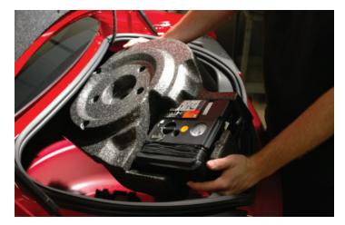
Use a 10mm wrench to loosen and then disconnect the negative (-) battery cable at the terminal. Cap or cover the terminal to protect against accidental contact with the battery post.
