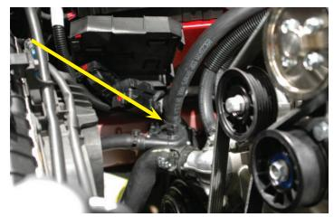
158. Route the hose up parallel to the heater hoses to the outlet barb of the intercooler reservoir. Clamp securely on the reservoir barb using a provided worm gear clamp. This may be made easier by removing the upper end of the fuel line hose to the manifold at the fuel rail temporarily.
