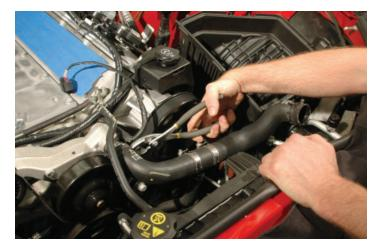
38. Disconnect the overflow hose from the radiator fill spout, pull free from the mounting clamps and wrap up around the overflow bottle cap out of the way.
