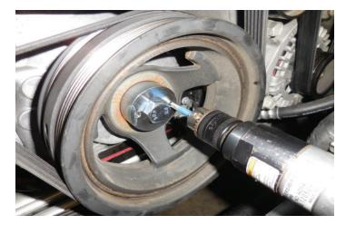
50. Place two provided pins into the holes. Use a drift pin, or nail set to ensure that the two pins get completely into the holes.
