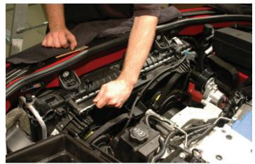
87. Plug the electrical connection back into the fan shroud assembly.
