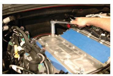
56. NOTE: L-99 cars or cars with Displacement On Demand (D.O.D.) will retain D.O.D. valley cover, skip to step #61. Damage to engine may occur if MagnaCharger valley cover is installed on D.O.D. equipped vehicles. Remove the eleven valley cover bolts using a 13mm socket and set aside.
