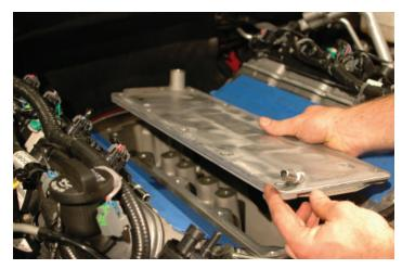
58. NOTE: L-99 cars or cars with Displacement On Demand (D.O.D.) will retain D.O.D. valley cover, skip to step #61. Damage to engine may occur if MagnaCharger valley cover is installed on D.O.D. equipped vehicles. Verify the integrity of the existing valley cover gasket, and that it is correctly positioned on the valley surface.
