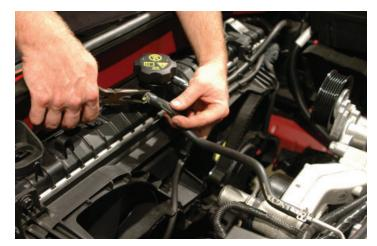
90. Pull the radiator upper hose from between the PS pump and air box, and relocate to the stock barbs on the water pump and radiator, re-attach the hose clamps to secure the hose to the hose barbs.
