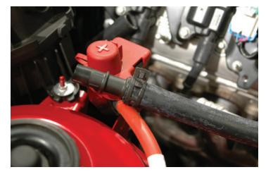
165. Route the remaining driver side intercooler heat exchanger hose up into the engine compartment toward the air conditioner hoses. Cut 2-1/2" off the hose end and using the provided clamp join the hose to the hose coupler just installed in the previous step. Use a zip tie to anchor the coupling to the existing battery wire loom bundle behind the air-box.
