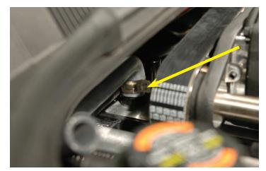
161. Cut 1" off of the remaining short leg of this hose and route to the intercooler reservoir. Use a provided worm gear clamp on the reservoir barb and tighten securely.
