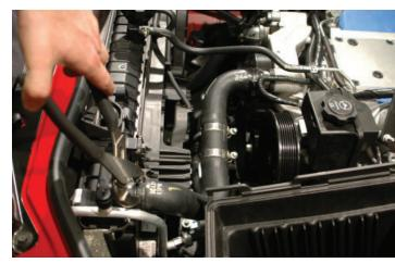
91. This is the provided Electronic Throttle control (ETC) connector extension harness.
