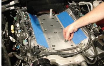
65. Replace the oil pressure sensor plug and locking clip on the oil pressure sensor.
