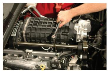
115. Attach the supplied MAP sensor extension harness to the existing MAP plug.
