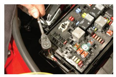
175. Zip tie the fuse holder of the wire harness to the existing wire harness by the headlight adjusting screw as shown.
