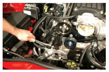
145. Install the supplied 76mm pulley and torque the bolt to 40 ft-lbs. Verify your torque wrench settings.
