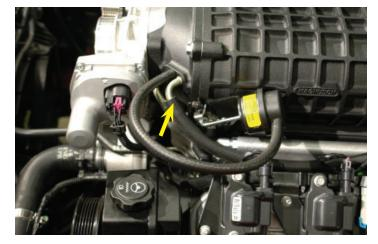
132. Cut a section of the supplied 11/32" brake hose to 30" in length. Attach the OEM check valve removed in step #106 to one end of this hose. NOTE: L-99 or D.O.D. cars; brake booster will have a sensor in place of the check valve. Install the hose onto the sensor instead. Sensor was removed from booster for ease of installation and photograph.
