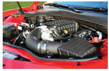
196. Test-drive the vehicle for the first few miles under normal driving conditions. Do not perform any wide open throttle runs. Listen for any noises, vibrations, engine misfire or anything that does not seem normal. The supercharger does have a slight whining noise under boost conditions, this is normal.
