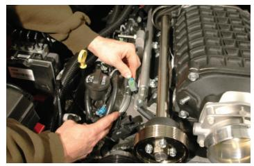
118. Re-mount the modified coil brackets to each side of the engine using the stock hardware. Torque all bolts to 106 in-lbs. Verify your torque wrench settings.
