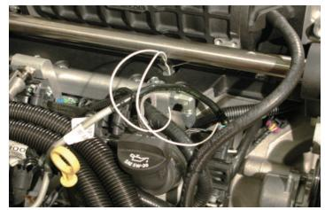
138. Crimp on a provided wire splice connector to each of these wire ends.
