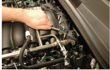
29. Unbolt the OEM intake manifold by removing the ten intake manifold bolts using an 8mm socket wrench; there are five on each side.
