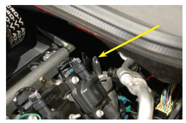
130. Cut a section of the 3/8" hose to 22" in length. Plug one end of this hose on this PCV valve barb just uncovered.
