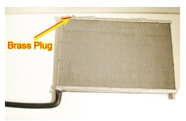
80. Cut 1-3/4" off the short side of the 3/4" x 4" x 36" x 90° angle hose. Use the supplied spring hose clamp to attach the short end of the hose to the remaining hose barb of the heat exchanger. This hose will also be pointing outward as shown.
