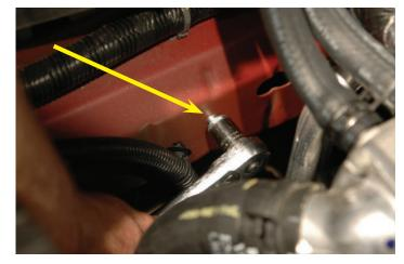
152. There are two ways to approach this. The first way: You place the Intercooler pump in the Adel clamp so that the bolt will be toward the rear. In all cases, the discharge barb points forward and directed toward the outside edge of the fan shroud. Tighten the bolt being careful not to strip the threads. The second way (pictured): Mount the Adel clamp to the frame but do not tighten. Use a mild soap solution (like Windex) to lubricate the rubber of the clamp.
