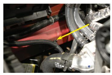
151. Use the provided self-tapping bolt and a ½" socket to prep the hole just vacated for mounting the intercooler pump. Chase the hole to ensure the proper bolt function.
