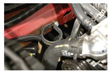
153. Slide the pump into the Adel clamp. Access to tighten the bolt is easiest if done from below.
