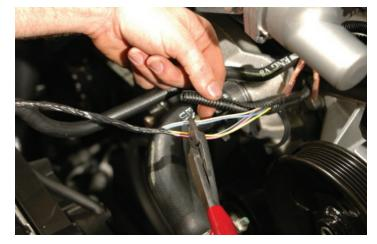
140. Pull these two wires out of the loom back to where the split-ring mount clamps to the hose barb at the water-pump. Tuck the two white wires from step #137 under the supercharger inlet and crimp one to each of the tan and blue wires. It doesn't matter which attaches to which.
