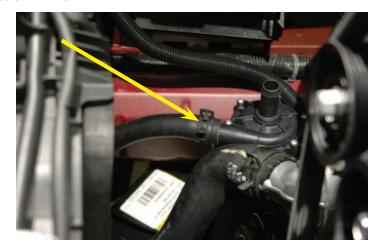
157. Take the cut-off section of the hose in the last step and attach one end to the inlet barb of the intercooler pump. Clamp on the barb with a provided spring clamp.
