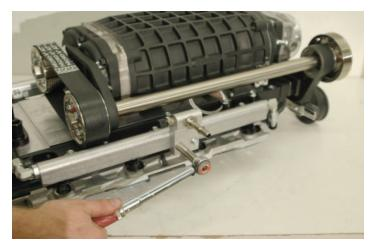
113. Remove the tape from the heads and lubricate with silicone spray, mildly soapy water spray, or a suitable lubricant (non-petroleum based to allow some sliding movement), get an assistant to help, and carefully lift the supercharger assembly into the engine.
