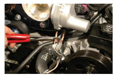
141. Use a heat gun or hair dryer set on high to shrink these connections securely. The ends of the blue and tan wires that go to the plug are abandoned and can be taped off and recovered with the existing split loom.
