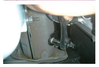
68. The heat exchanger (LTR-being installed in the upcoming steps) will be shifting about 3/4" toward the passenger side of the vehicle. The air deflector will need to be modified slightly to create access for the heat exchanger hose barbs. The existing notches will need to be increased about 3/4" toward the passenger side of the vehicle on each side of the air deflector as shown by this driver side tape application.
