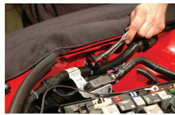
178. Cut the existing "eyelet" connector off the black ground (-) wire, strip off ½" of the insulation and crimp on the supplied larger "eyelet" connector.
