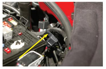
176. Route the intercooler pump plug around the fuse center and down toward the intercooler pump. Plug the end into the terminal at the bottom of the intercooler pump.
