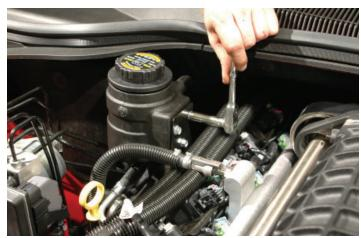
156. Route the passenger side hose from the intercooler heat exchanger up into the engine compartment. Cut the hose to fit at the intercooler pump discharge barb. Clamp on using a supplied spring clamp. Save the cut section of hose for the next step.
