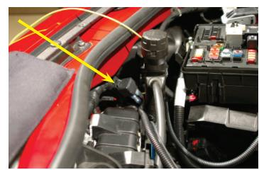
174. Replace the positive (+) lug nut incorporating the red wire "eyelet" you attached in step #172 from the new harness.
