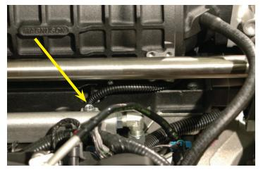
144. Use a 15mm wrench to remove the OEM tensioner pulley.
