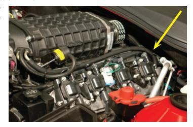
137. On the passenger side of the Supercharger assembly, near the front are two white wires exiting the intercooler lid. These are the IAT sensor wires. Strip off about 3/8" of the insulation on each of these wires.
