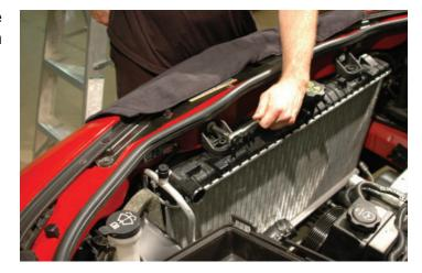
86. With the radiator mounted back in the stock location, use a 13mm wrench and the stock hardware to re-install the electric fan shroud assembly.
