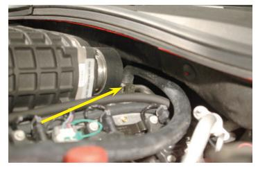
164. Cut 11" off the end of this hose and route below the air conditioner hose bending toward the front of the vehicle. Insert the provided hose coupler and use the provided clamp to prepare the end of this hose.
