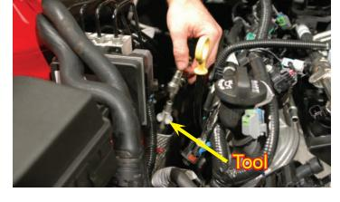
28. Remove the engine cover hold down bracket using a 10mm wrench on the driver side near the end of the fuel rail. Then pivot the hold down bracket up and pull free from the engine. This will not be reused.
