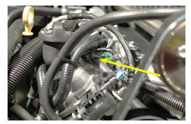
189. Route the other end of the hose behind the pulleys and push onto the hose barb on the bottom of the air inlet tube assembly, in front of the throttle body.
