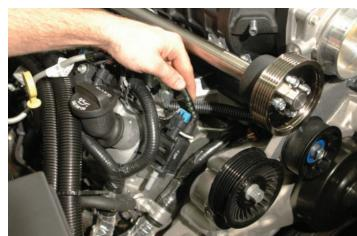
126. Use a sharp blade and carefully split the end of the EVAP tube (removed in step #22) to salvage the 90° fitting.
