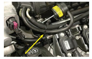
136. Add a zip tie to loosely tie the brake booster hose and the PCV hose together where they meet at the rear of the engine.
