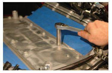
57. NOTE: L-99 cars or cars with Displacement On Demand (D.O.D.) will retain D.O.D. valley cover, skip to step #61. Damage to engine may occur if MagnaCharger valley cover is installed on D.O.D. equipped vehicles. Remove the OEM valley cover. This will not be reused, but we will need components from it.
