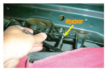
70. **NOTE:** All vehicles continue from here: Remove the two upper radiator mounting bolts using a 10mm socket wrench.
