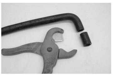
163. Place a provided clamp on the short leg of this hose and push the end onto the intercooler barb on the driver side behind the supercharger. Tighten the clamp securely with the hose pointing toward the driver side of the vehicle.
