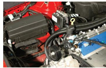
103. Remove the MAP sensor from the OEM intake manifold using a T-25 Torx wrench.
