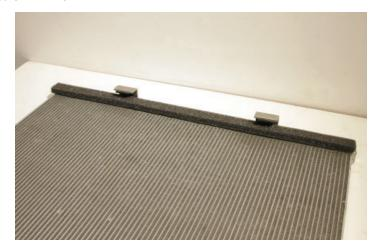
78. Attach the other strip to the inside-bottom edge of the heat exchanger as shown.
