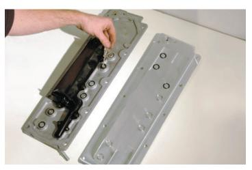
60. NOTE: L-99 cars or cars with Displacement On Demand (D.O.D.) will retain D.O.D. valley cover, skip to step #61. Damage to engine may occur if MagnaCharger valley cover is installed on D.O.D. equipped vehicles. Install the new valley cover using the eleven provided Allencountersunk bolts. Torque to 18 ft-lbs using a 5mm Allen socket. Verify your torque wrench settings.
