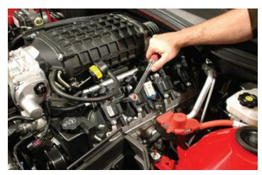
119. Plug in the main coil connectors on both sides of the engine.
