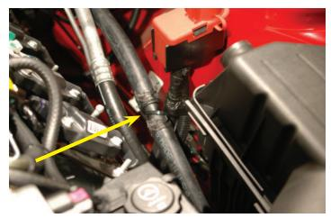
166. Slide a length of the provided 1" split loom over the passenger side intercooler heat exchanger hose to protect the hose from chaffing at the rectangular hole in the splash shield and adjacent edges.
