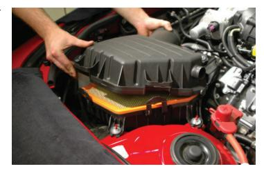
149. Plug the MAF sensor connector at the airbox neck.
