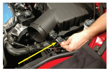
35. Release the two clips on the air-box cover.
