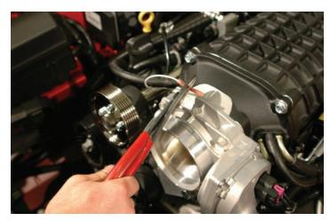
139. Uncover the MAF wire loom connector that hooks to the air box. This should be by the upper radiator hose at the water-pump. Cut the blue and the tan wire even with the end of the existing wire loom. Strip off about 3/8" of insulation from the end of the two wires that continue back in the split loom toward the engine.
