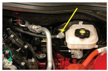
134. Route the hose just below the PCV hose between the fuel rails and coil bracket and attach the loose end to the front barb on the Supercharger inlet.
