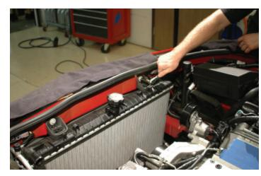
71. Remove the two upper radiator mounting brackets.
