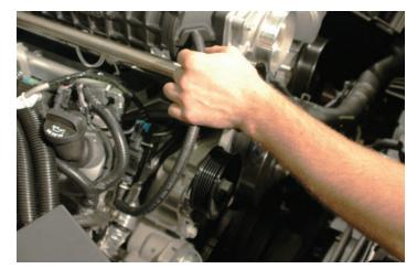
129. On the driver side of the engine, at the rear of the valve cover, adjacent to the fuel rail crossover and the coil bracket is a PCV hose barb covered with a cap. Remove this cap. NOTE: L-99 or D.O.D. vehicles will not have this cap and instead will have a PCV hose connection here.
