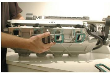
111. Using the provided Lubriplate lubricant, lube the fuel manifold O-ring and insert it into the groove on the passenger side fuel rail.
