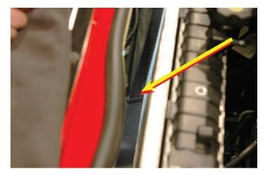
82. With the help of an assistant, guide the two hoses through these holes. From below pull on these hoses while the assistant holds the radiator pushed back and guides the heat exchanger down in front of the existing radiator and AC condenser assembly.
