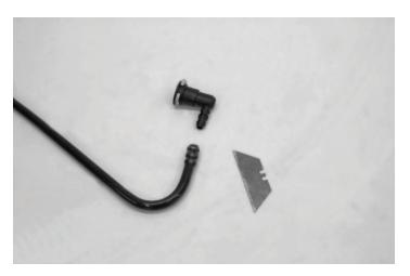
127. Cut a 15" piece of the supplied 5/16" hose and install the right angle fitting just removed in the last step.
