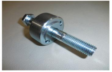
45. Replace the removed crank pulley mounting bolt with the provided drill guide and mounting bolt. It's easier if you have the holes of the drill guide oriented horizontally for visibility purposes. Torque this down to 24 ft-lbs.
