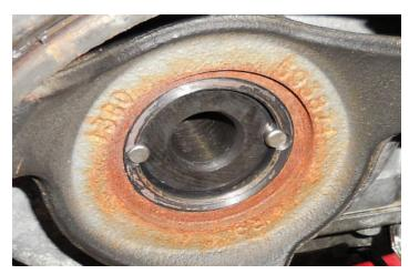
52. Install the new provided factory GM harmonic balancer bolt. Using a 24 mm socket, tighten the new harmonic balancer bolt according to the GM specifications. a. Tighten to 50 N-m (37 ft-lbs) using a torque wrench. Verify your torque wrench setting. b. Tighten an additional 140° using a torque angle meter.
