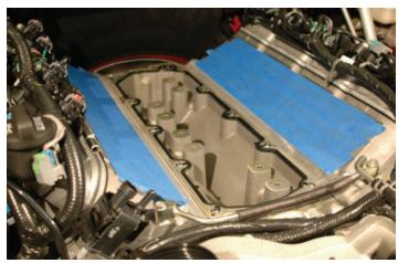
59. NOTE: L-99 cars or cars with Displacement On Demand (D.O.D.) will retain D.O.D. valley cover, skip to step #61. Damage to engine may occur if MagnaCharger valley cover is installed on D.O.D. equipped vehicles. Remove the existing O-ring seals from the OEM valley cover, and place in the O-ring grooves of the new provided valley cover.
