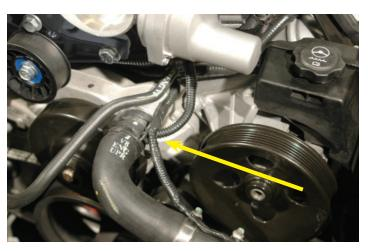
143. The other end should reach all the way to the other end of the wires at the Supercharger lid. It's a good idea to cross tape the junction of the two split looms at the water-pump hose barb.
