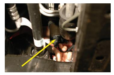
177. Use one of the provided self tapping bolts and a ½" socket to tap the hole in the fender well just forward of the shock tower and above the existing wire loom as shown.
