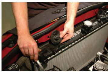
72. Pry off the rubber deflector strip from the top/ front of the radiator. Put these parts aside for later reinstallation.
