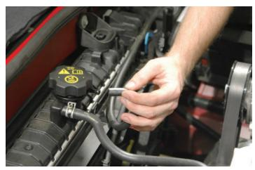
39. Disconnect the steam vent hose from the radiator fill spout, and tuck this behind the power steering pump.
