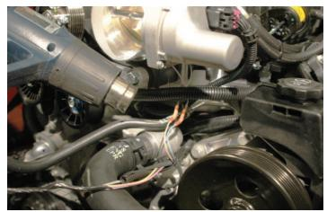
142. Cut a piece of the provided split loom (about 18") to reach from the split-ring clamp, following the white wires back to where they enter the Supercharger lid on the passenger side of the Supercharger. Slide the split loom over the wires, one end should be at the junction by the split-ring clamp.
