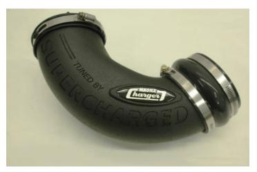
187. Push the air inlet tube onto the air-box and throttle body necks and tighten all clamps securely.
