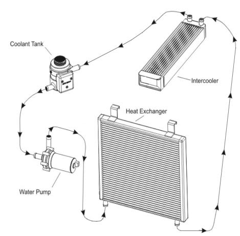
**Intercooler Routing Diagram**
