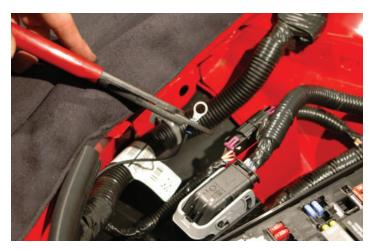
179. Use the self tapping bolt from two steps ago, incorporate the just installed "eyelet" on the black wire from the last step, and ground the wire harness to the automobile body at the prepped hole. Tighten snugly being careful to not strip the threads.
