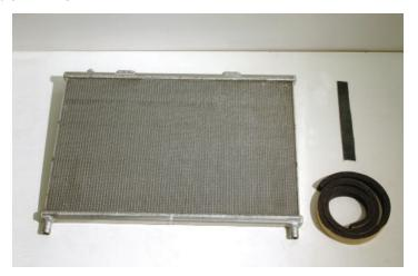
74. Cut the strip of the supplied adhesive backed foam in half
