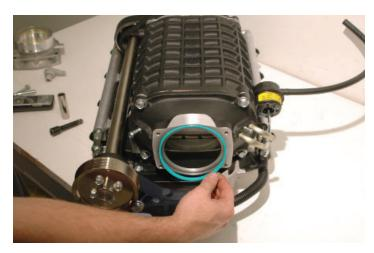
108. Install the OEM throttle body onto the supercharger inlet using a 10mm socket wrench. Torque the bolts to 106 in-lbs. Make sure you are using the correct settings on your torque wrench.
