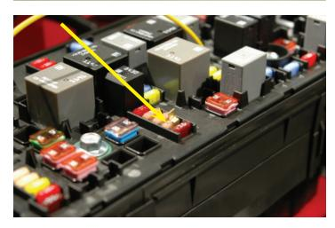
183. Strip off 3/8" of the insulation off the end of the yellow wire and crimp on the provided spade connector.
