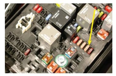
181. Install the provided fuse-tap on one leg of the fuse.
