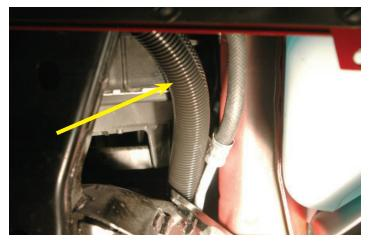
168. These are the intercooler pump wiring harness components.
