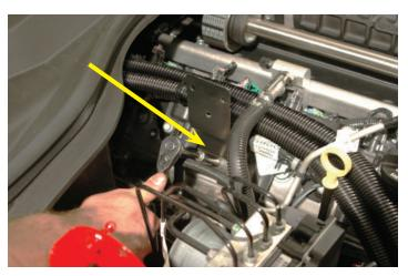
155. Attach the reservoir bottle to the bracket as shown with the supplied bolts and a 10mm wrench.
