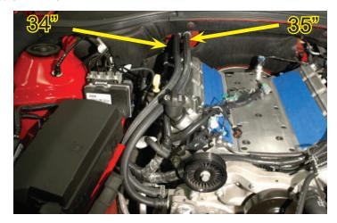
102. Cut two pieces of the supplied split loom to cover these hoses as they pass by the existing fuse center mounting platform and over the valve covers.
