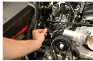
23. Unplug the remaining EVAP hose that goes from the sensor to the hard-line fitting on the passenger side. Tuck aside near the brake module for later reinstall.
