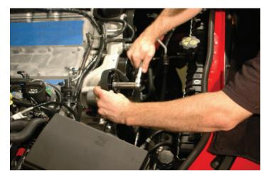
54. Unplug the oil pressure sensor from the back, driver-side of the OEM valley cover.
