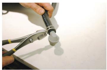
107. Install the O-ring just removed from the manifold into the groove on the supercharger inlet.
