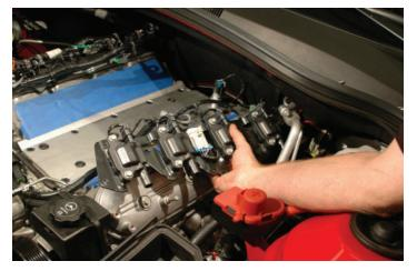
97. The plastic wire loom covers from the coil bracket assemblies must be removed. Unsnap the connecting clips and remove from both sets of coil brackets.
