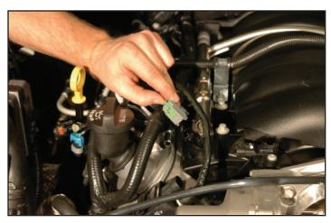
20. Unplug the electronic throttle body connection.
