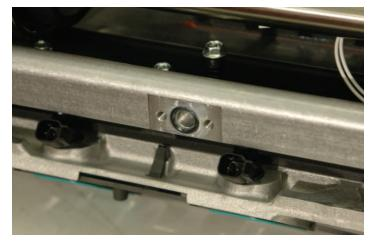
112. Install the fuel supply manifold on the fuel rail and torque to 106 in-lbs. Verify your torque wrench settings.
