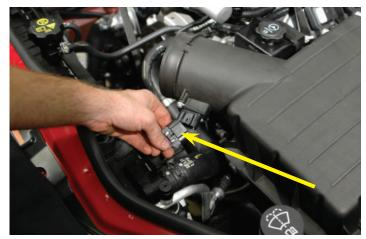
150. On the passenger side of the engine, near the thermostat on the frame rail, unplug the fuse center wire loom hold-down clip by pulling it away from the frame.
