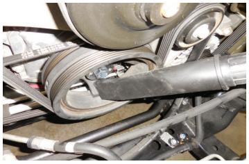
49. Install the reamer bit in your drill motor and ream out your holes. Once again use compressed air to remove debris from the two holes. Now remove the drill key way guide and mounting bolt using a 22mm socket.
