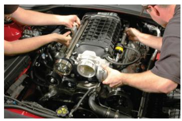
114. Remove the split loom spacers from the pre-installed manifold bolts and after an initial hand tighten using a 10mm socket, torque the bolts down to 106 in-lbs using a cross rotation pattern. Make sure to verify your torque wrench settings.
