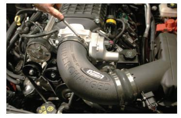
188. Cut a piece of the remaining 3/8" hose to fit between the PCV fitting on the passenger side valve cover near the oil-fill spout, and the hose barb on the bottom of the air tube assembly. Push one end onto the hose barb at the front of the valve cover.
