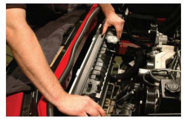
85. Reinstall the upper radiator clamps using the stock hardware and a 10mm wrench. Tighten securely.
