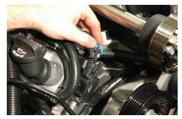
125. Plug in the 90° fitting of the EVAP tube (from the hard-line on the passenger side running over the heater hoses) to the upper EVAP solenoid barb.
