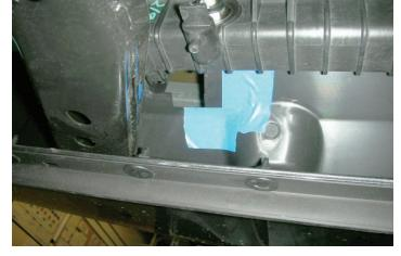
69. Once your notches are complete, reconnect the top "A-frame" bracket using the provided longer bolts, incorporating the provided spacer between the "A-frame" and the upper cross frame fascia support. Tighten all your bolts and torque to 40 ft-lbs. Verify your torque wrench settings.
