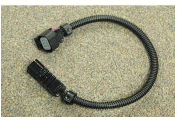
92. Locate the ETC connector on the OEM engine harness. Plug the extension harness into the existing ETC connector and route adjacent to the steam pipe to the driver side of the engine.
