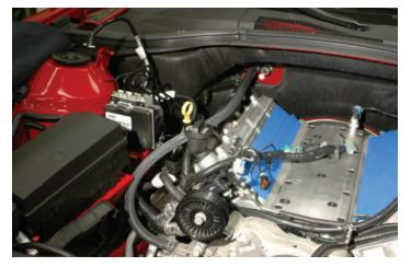
101. Use the 35" x 3/4" hose and the removed clamps to attach to the remaining barb on the water-pump. Route the other end parallel to the just installed hose and connect to the remaining hose barb at the firewall using one of the removed clamps.
