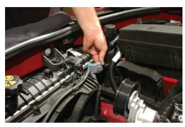
88. Uncoil the coolant overflow from the reservoir bottle, and relocate through the stock clip locations. Re-connect the coolant overflow hose back onto the hose barb on the radiator neck.
