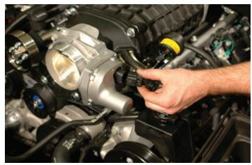
122. Attach the supplied fuel line between the fuel supply barb below the ABS Module (where the OEM fuel line was disconnected in steps # 26-27) and the new fuel rail manifold on the passenger side of the vehicle. Pull firmly on both ends to verify that you have a good connection. The EVAP sensor tube should be under the fuel line and above the heater hoses. IMPORTANT: You should NOT be able to remove the fuel line from either end without the use of the fuel line removal tool.
