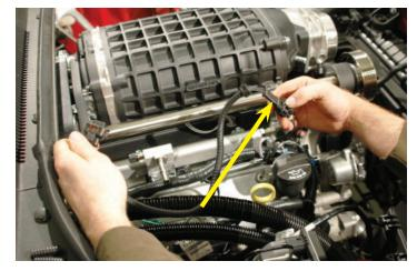
116. Plug the other end of the extension harness into the MAP sensor located under the rear fuel rail cross-over tube at the back of the passenger side of the engine.
