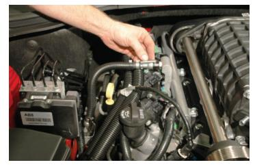
124. Plug in the EVAP solenoid electrical connection at the front of the passenger side valve cover.
