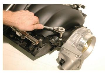
104. Use a 10mm socket wrench to unbolt and remove the throttle body from the OEM intake manifold.
