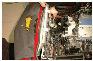
83. Guide the "hooks" of the intercooler heat exchanger over the top of the AC Condenser. Ensure that the foam is between the two (both top and bottom), and the rubber strips are still in place around the "hooks".
