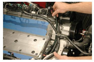
93. Disconnect the main coil connectors from the center of the coil rails on both sides of the engine.
