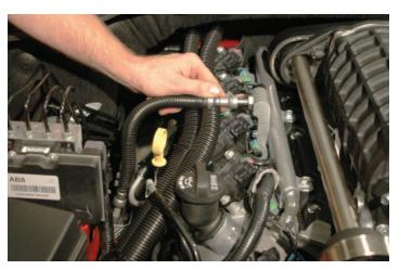
123. Remove the fuel line safety clip from the fuel line still attached to the OEM intake manifold. Use this and the clip removed in step #26 to re-attach fuel line safety clips on both ends of the fuel line.
