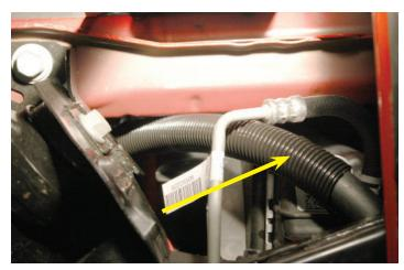
167. Slide a length of the provided 1" split loom over the driver side intercooler heat exchanger hose to protect the hose from chaffing at the rectangular hole in the splash shield and adjacent edges.
