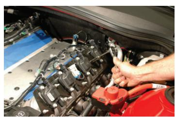
96. Remove the coil brackets from the mounts on the rocker covers on both sides and put on a bench for some required modifications.
