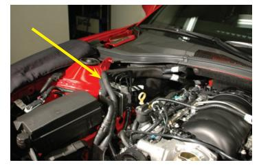
17. Disconnect the EVAP solenoid electrical connector.
