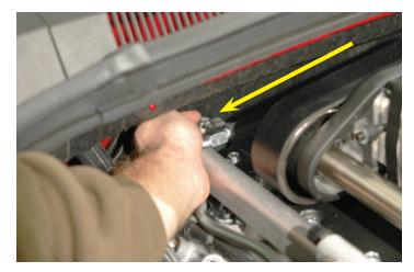
117. Plug in the fuel injector connections to the injectors on each side of the engine. Make sure to route and stuff the wiring to avoid moving components.
