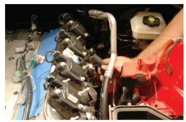
95. Use a 10mm wrench to remove the five bolts from the coil brackets on each side of the engine.
