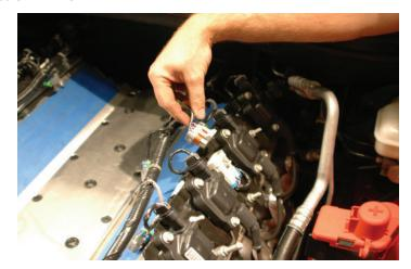
94. Disconnect all plug wires from the coils on both sides of the engine.
