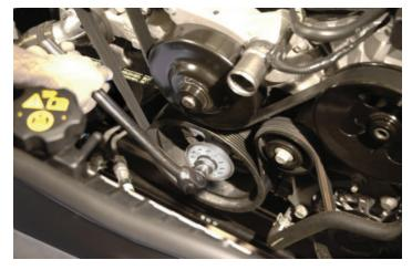
53. Using a 15mm socket on the Tensioner Pulley bolt, spring the pulley down to remove tension on the drive belt and remove the belt when tension has been released.
