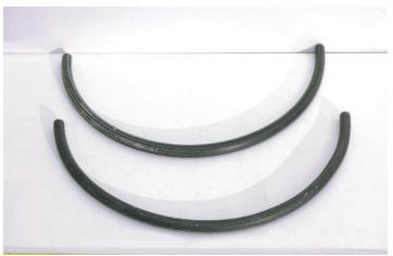
100. Take the 34" x 5/8" hose and use one of the clamps removed to attach the hose to the smaller barb at the water-pump. Route the other end up between the oil fill spout and dipstick. Use one of the removed clamps to connect the hose to the smaller barb (outside) on the firewall.
