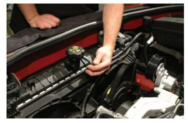
89. Reconnect the steam vent hose to the barb at the side of the radiator neck; place the stock clamp back in position.
