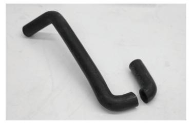
160. Use a provided spring clamp on the end of the hose you just cut and push the remaining section of the "U" onto the passenger side barb of the intercooler. Verify your hose is secure and the hose is pointed toward the passenger side of the car as shown.
