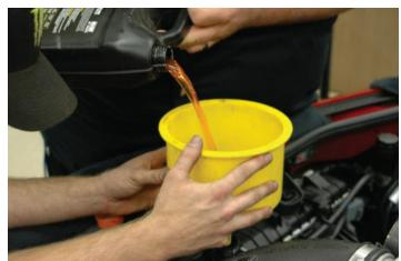
194. Fill the Intercooler System with the vehicle manufacturer recommended coolant mixture. Have an assistant temporarily key vehicle on to accessory mode (Do Not start the vehicle) to turn the pump on. Key vehicle off after 5 seconds. Fill reservoir full again and continue this process until fluid is circulating. At this time check your intercooler system, and fuel system for leaks.
