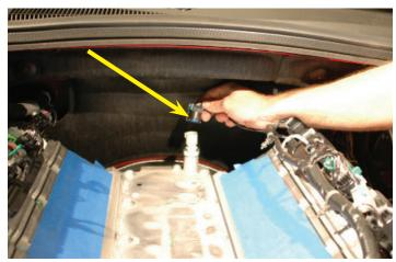
55. NOTE: L-99 cars or cars with Displacement On Demand (D.O.D.) will retain D.O.D. valley cover, skip to step #61. Damage to engine may occur if MagnaCharger valley cover is installed on D.O.D. equipped vehicles. Remove the oil pressure sensor from the valley cover using a 6-point 1-1/16" socket or wrench, put aside for later re-installation.
