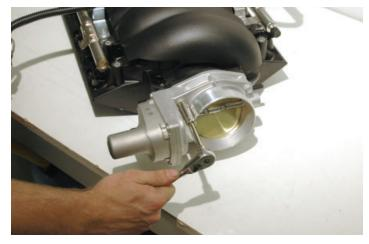
105. Remove the O-ring from the stock throttle body connector groove.
