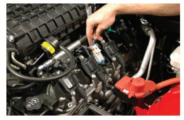
120. Attach the stock plug connectors back onto the coils on the coil brackets on both sides of the engine.
