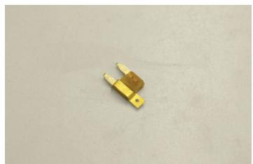
182. Replace the IGN fuse with the fuse tap back into the slot from whence it came.
