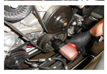
44. This is the pin drill guide and provided mounting bolt. The stepped side faces towards the crank to center with the pulley.
