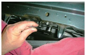
67. Loosen the 13mm bolts securing the bottom of the "A-frame" member to the frame rails on each side of the vehicle.
