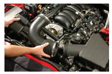
14. Rotate the passenger side vent tube removed from the air inlet in and earlier step to expose the release tab. This will be at the front of the passenger side valve cover adjacent to the oil fill spout. Spread the tab to release from the hose barb and remove the hose. This will not be reused.
