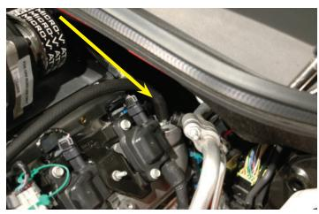
131. Route this hose along the fuel rail forward to the closest barb on the driver side of the Supercharger inlet.
