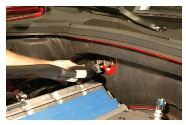
99. Cut the supplied 5/8" hose into a 34" length, and the supplied 3/4" hose into a 35" length if they are not already sized correctly.
