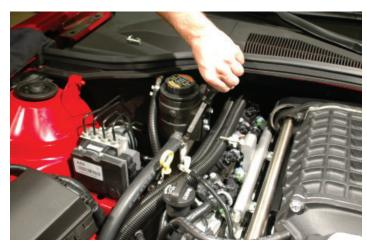
159. Cut off the "U" section short leg of the provided "J" hose. The short end will not be used.
