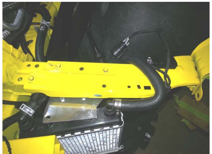
New Radiator Hose Routed
