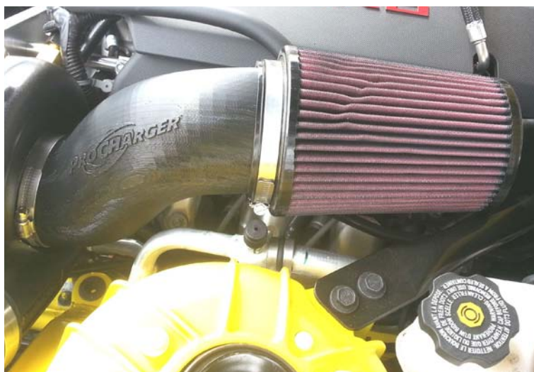
Air Inlet Installed
