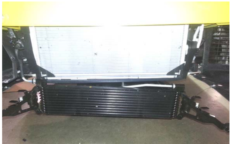
Transmission Cooler Dropped Down
