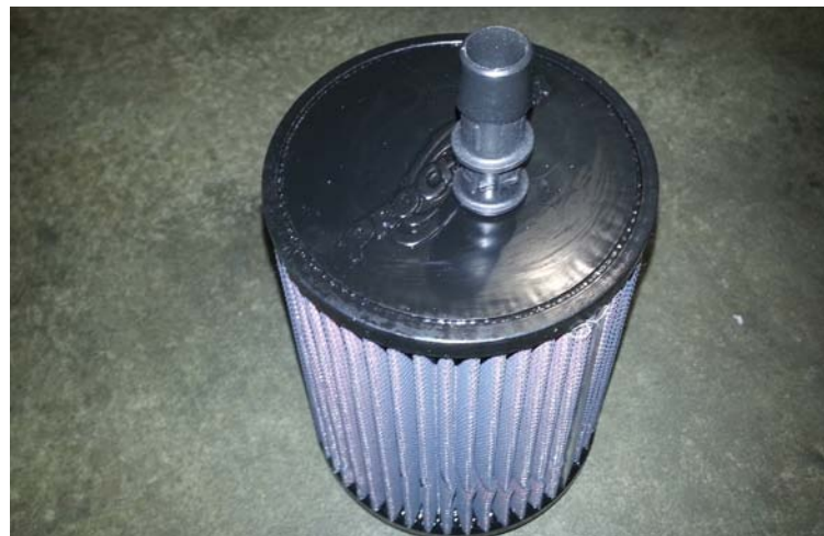
Plastic Fitting Installed in Air Filter
