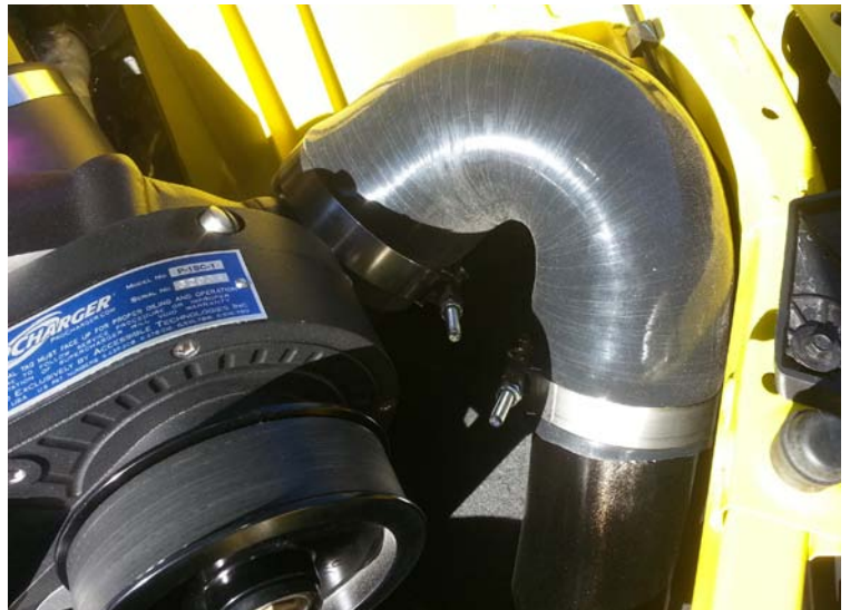
Blower Discharge Tube Installed
