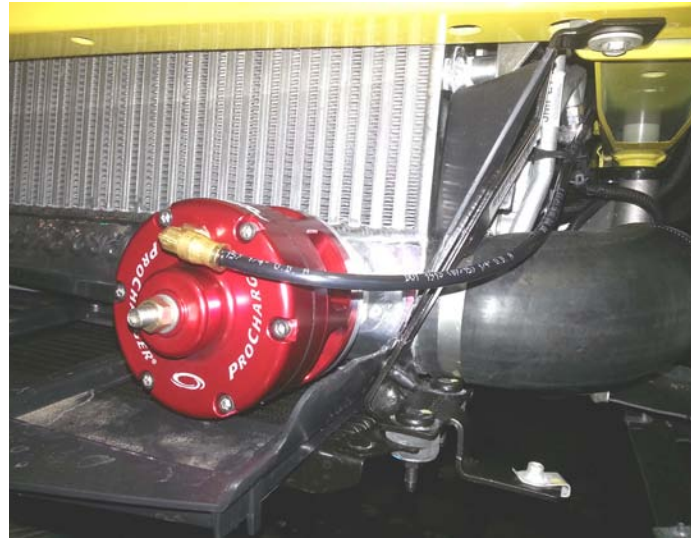
Race Valve Installed
