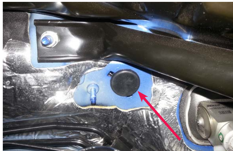
Firewall Plug Installed
