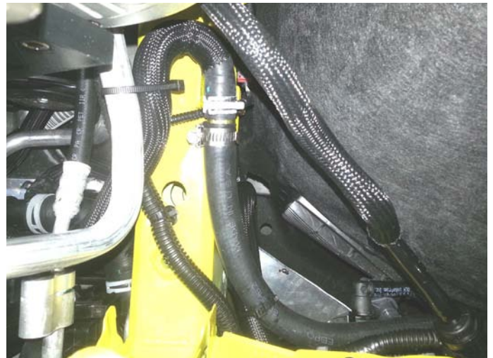
New Hose Connected to Factory Hose
