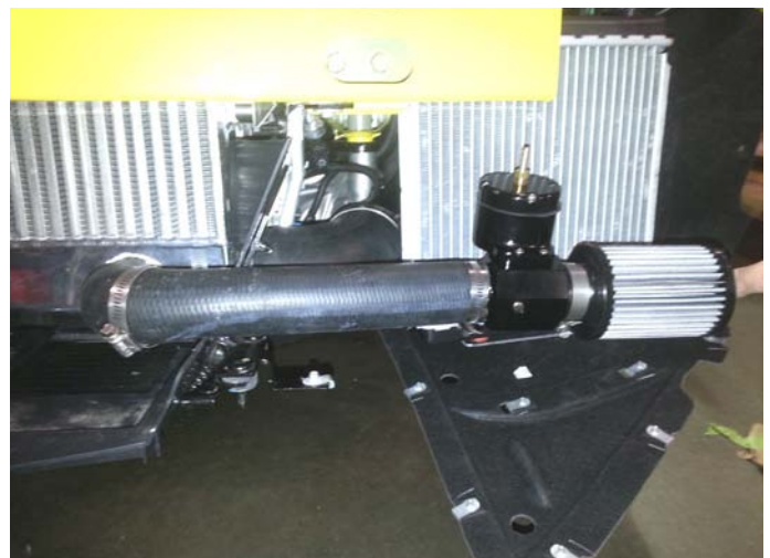
Proflow Surge Valve Installed
