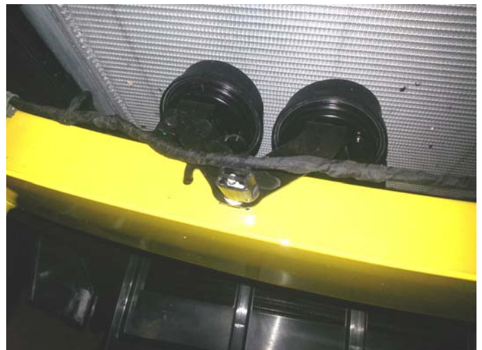
Factory Horn Location
