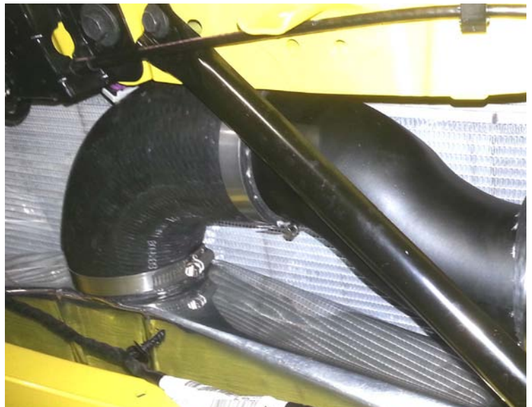
Tube #316 Installed (H.O. Intercooler Only)
