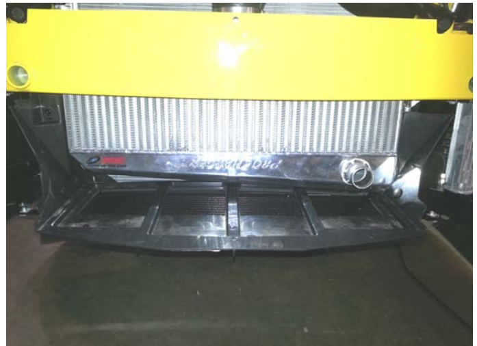
Modified Air Shroud Installed
