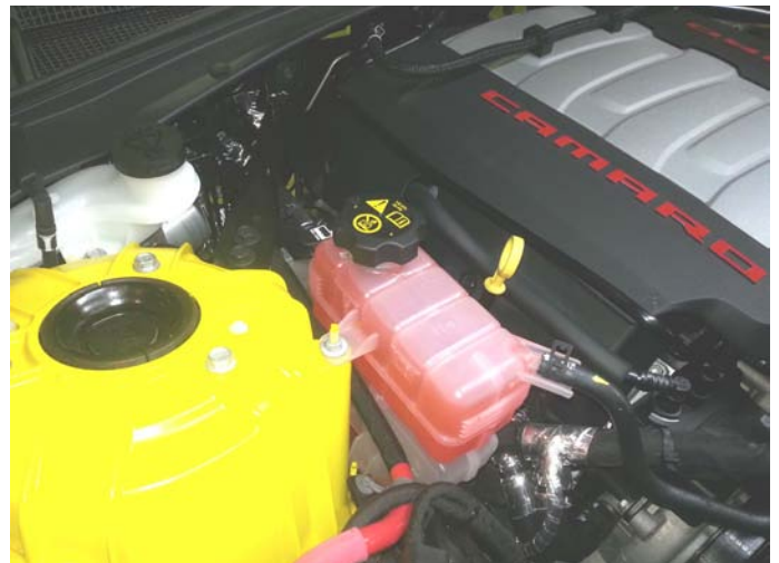
Cooling System Refilled
