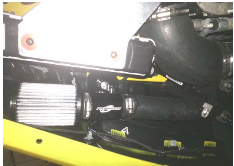
Surge Valve After Fascia Installation
