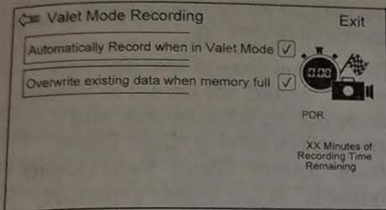
**Valet Mode Recording** : Allows recording preferences to be selected. It is recommended that a blank SD card be used. Available choices are:
