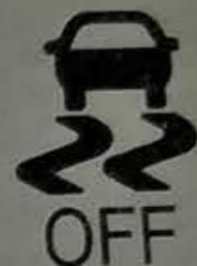
These lights are on when the vehicle is in PTM Mode.
