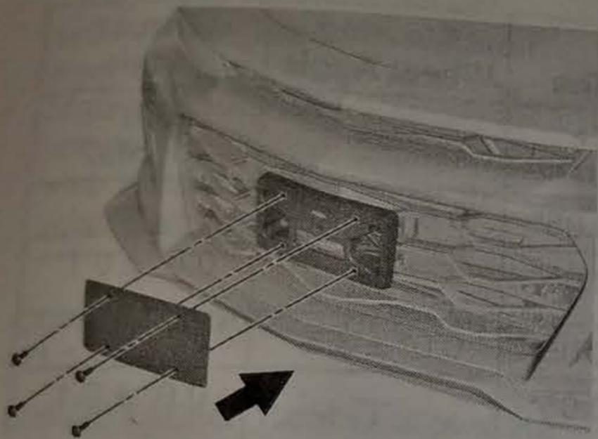
For track usage, the front license plate and bracket can be removed from the fascia for increased airflow. Remove the license plate to access the four screws that attach the license plate bracket to the front fascia.
