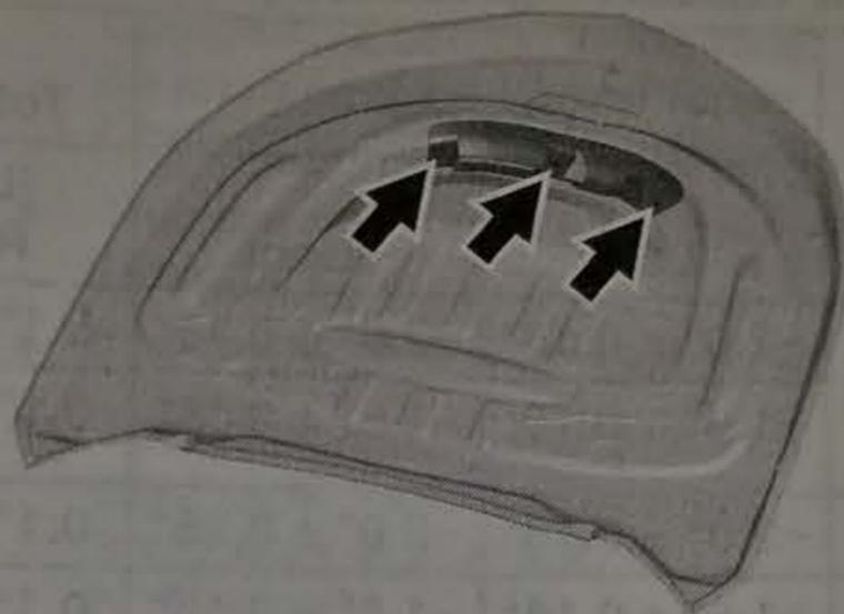
If operating a ZL1 on a closed course in hot temperatures, remove the water deflector to increase airflow and improve cooling. Remove the three bolts. Replace immediately after track use to protect the engine compartment from water intrusion. Torque to 4.5 N•m (40 lb in).
