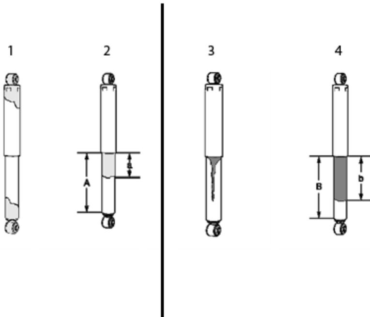
**Do Not Replace shock absorbers** displaying condition 1 or 2 levels of seepage.
