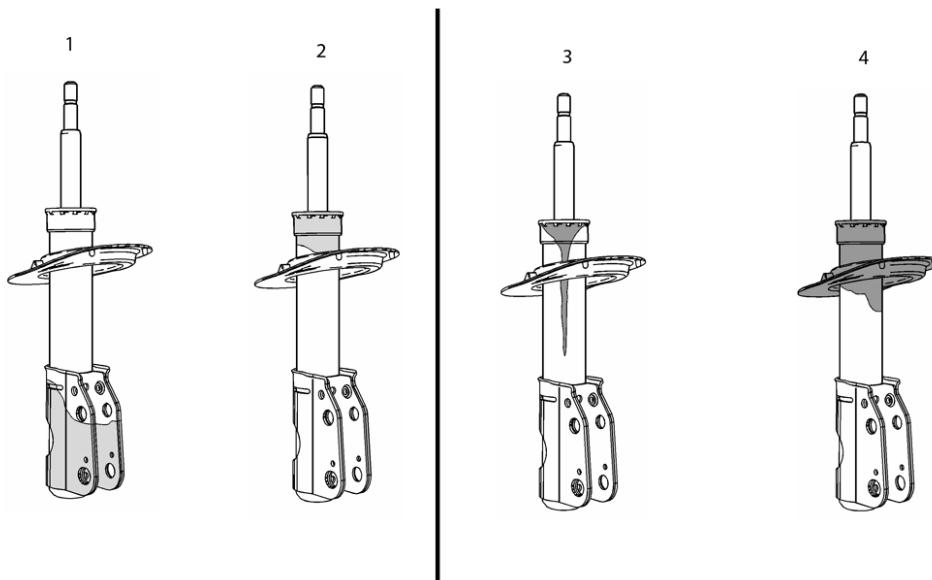
**Do Not Replace Struts** displaying condition 1 or 2 levels of seepage.
