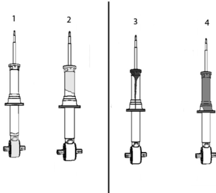
**Do Not Replace coil-over shock absorbers** displaying condition 1 or 2 levels of seepage.
