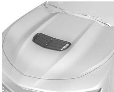
Hood Air Extractor
