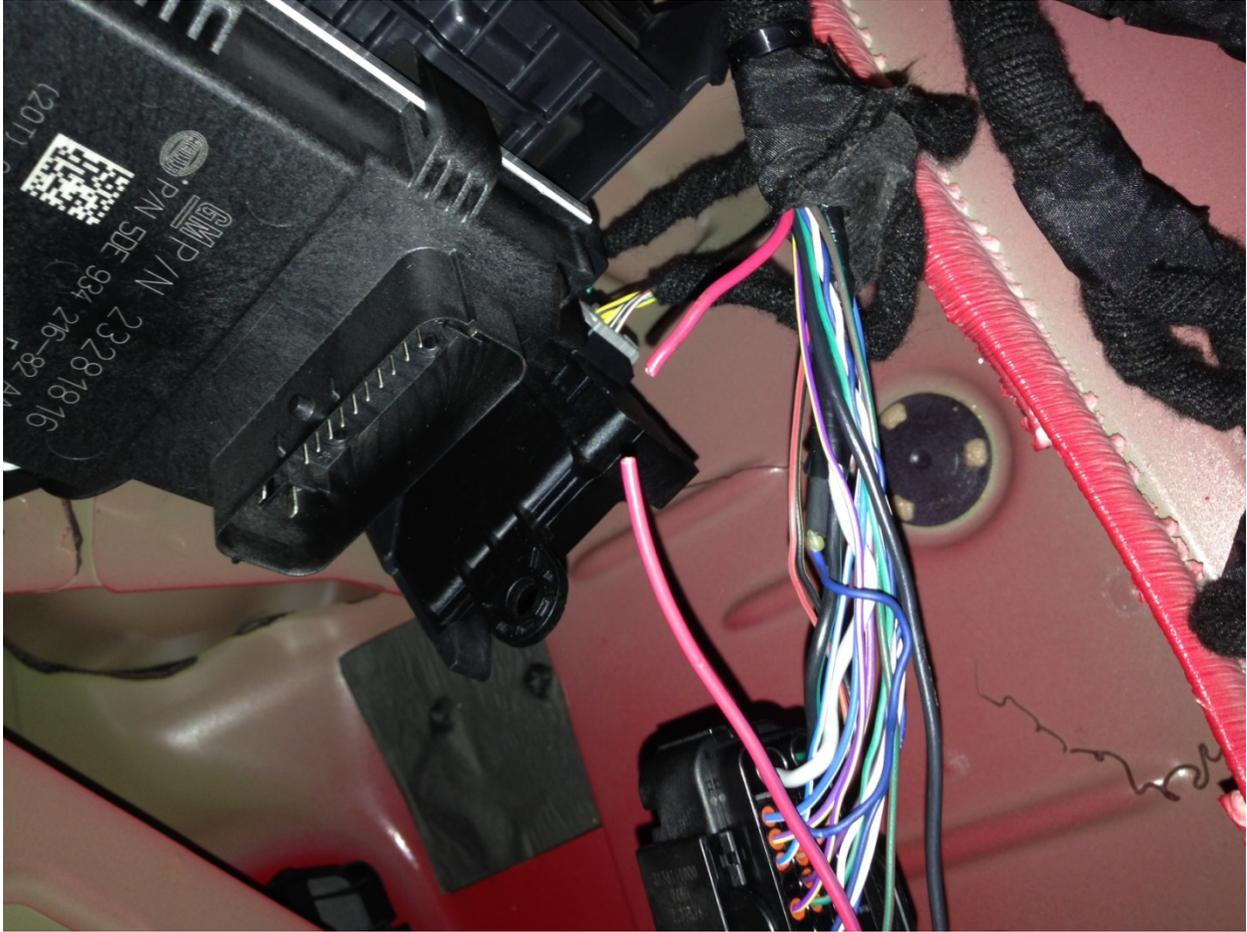
*Peel back wire covering. Undo clip from FPCM. Cut the large red with purple tracer.*
