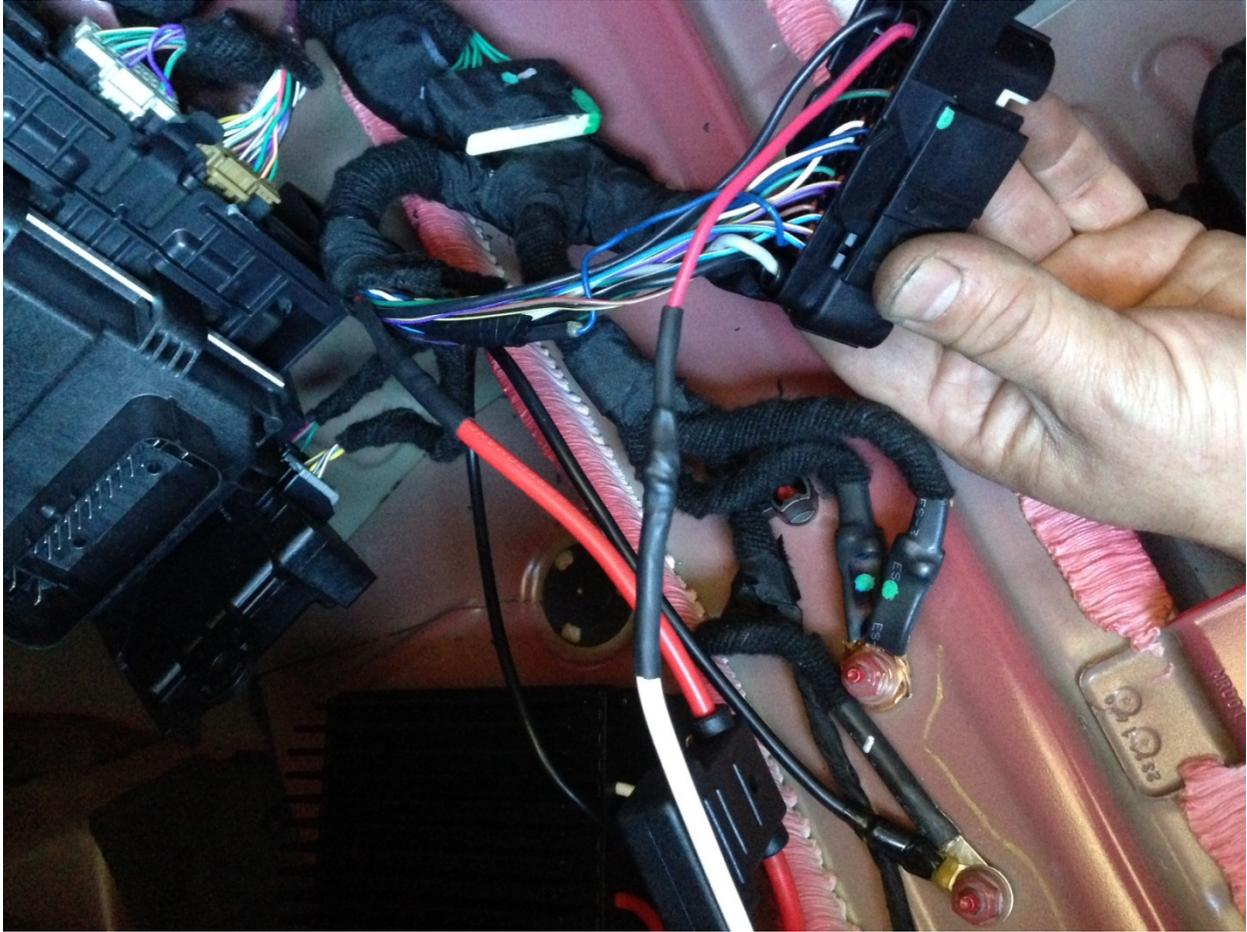
*White wire from JMS goes to the connector. Red Wire will go back to harness. Note black ground wire shown mounted to the body.*
