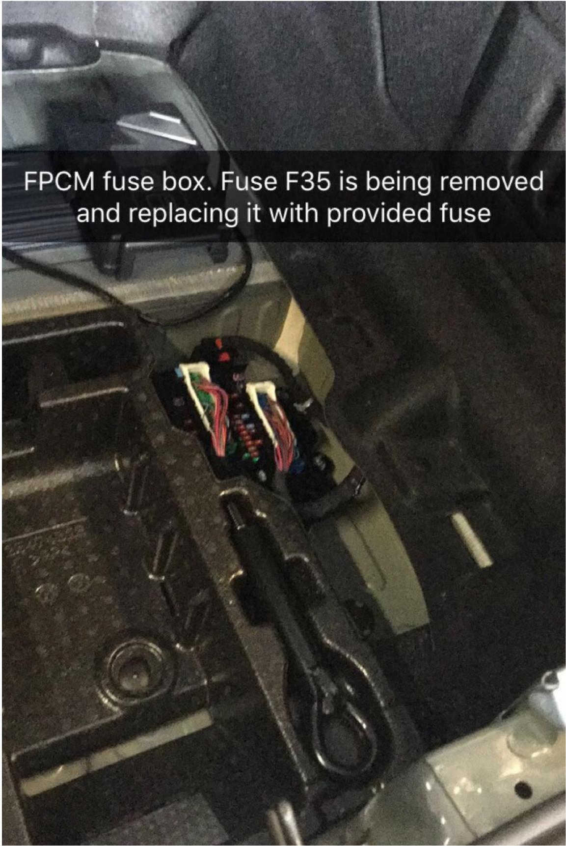
FPCM fuse box. Fuse F35 is being removed and replacing it with provided fuse
