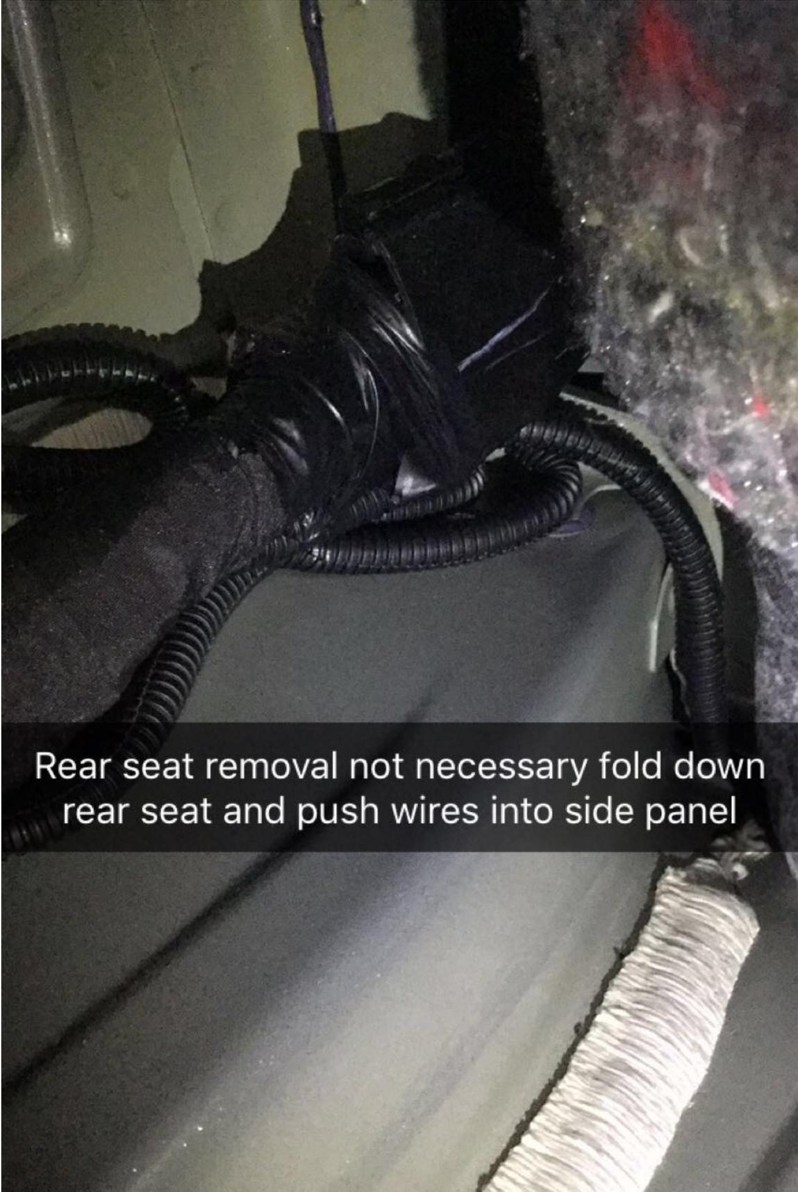
Rear seat removal not necessary fold down rear seat and push wires into side panel
