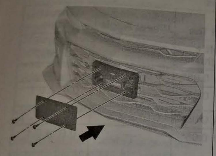
For track usage, the front license plate and bracket can be removed from the fascia for increased airflow. Remove the license plate to access the four screws that attach the license plate bracket to the front fascia. If operating a ZL1 on a closed course in hot temperatures, remove the water deflector to increase airflow and improve cooling. Remove the three bolts. Replace immediately after track use to protect the engine compartment from water intrusion. Torque to 4.5 N•m (40 lb in).
