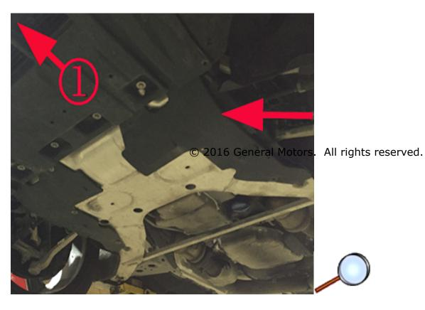
Pan part number will be about 6" behind the crank pulley, just rearward of the first "step up" surface. Wiring loom may need to be pushed aside to view.
