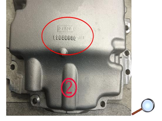
If the pan has raised marking in this location the pan will need to be repaired (see repair procedure). If markings are not present vehicle is good and can be released.
